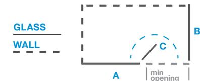
A: Front Panel B: End Panel C: Swivel Panel
