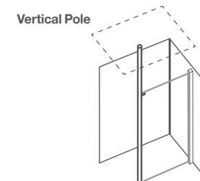
Supplied with high level vertical post. Post supplied 3 metre maximum length (designed to be adapted to size). Recommended opening min 500mm.
